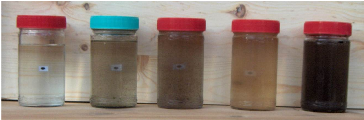
Figure 13. Turbidity of water samples from streams after the Power Fire of 2004, Eldorado National Forest.
